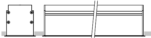
Frame recessed version / incasso con cornice variable lengths(L) x 88(W) x 87(H) mm
